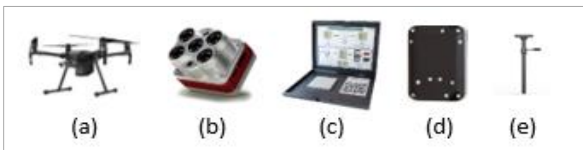
Figure 1. Unmanned aerial vehicle (a), Multispectral camera (b), Calibration plate (c), light sensor /DLS/ (d), Mobile GPS (e)
