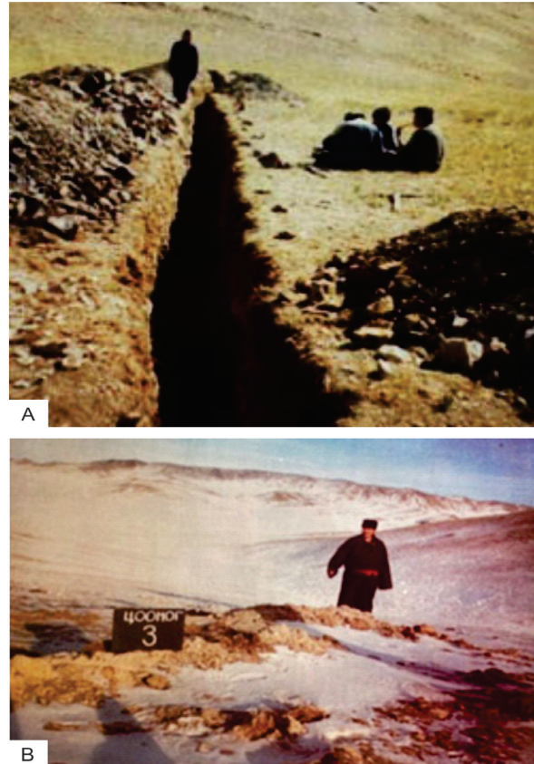
Figure 6. A. Tsakhir Uul deposit, location of prospecting trench № 8, length 45m, depth 3 m, ore thickness 12-40 m. B. Alagiin Davaa deposit, location of test pit № 3, depth 44 m.
