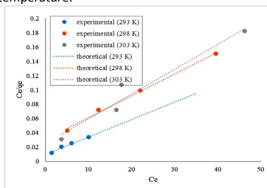
Fig. 6. Linear form of Langmuir isotherm model, experimental condition: pH= 6.0, room temperature 293 K
