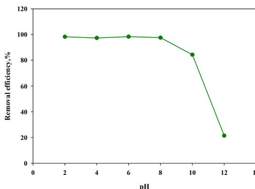
Fig. 2. Effect of pH on the sorption of reactive blue 50 ( $C_0=150 \text{ mg}\cdot\text{L}^{-1}$ , sorbent mass: 0.5 g)
