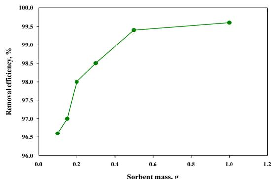
Fig. 4. Effect of sorbent mass on the adsorption of reactive blue 50 onto zero valent iron ( $C_0=150 \text{ mg}\cdot\text{L}^{-1}$ ,  $pH=6.0$ , room temperature)
