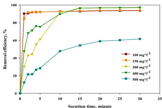
Fig. 3. Relationship between sorption capacity and sorption time ( $pH=6.0$ , sorbent mass:  $0.2 \text{ g}$ , room temperature)
