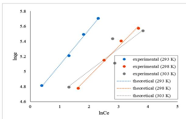
Fig. 5. Linear form of Freundlich isotherm model, experimental condition: pH= 6.0, room temperature 293K
