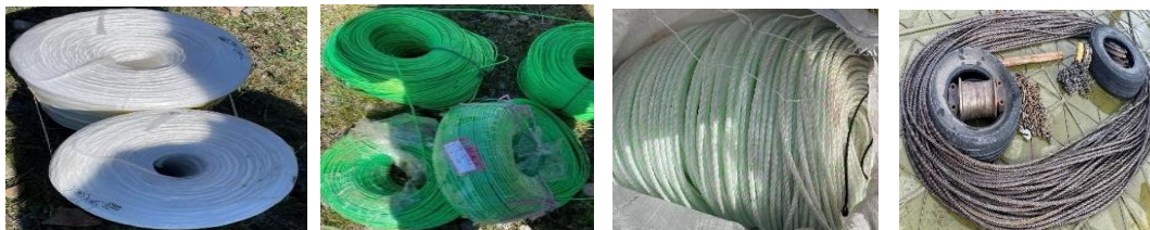
Figure 3. Fiber, flexible coated green wire rope, fiber rope, and steel wire rope used during threading
