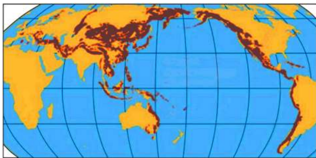
Fig. 7. Generalized overview of the global distribution of porphyry copper (modified after Dicken et al., 2016). The linear bands can be associated with unloading from deep fault zones, but the broad ore belt across the thick crust of Central Asia requires a different approach.
